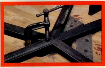
The Pusher's smooth lines and precision fittings are due in large part to computer-aided design and manufacturing (CAD/CAM). Fuselage framework is cut to fit with the help of computer-programmed saws, then hand-welded. Main gear trunnions (bottom right) also come pre-built. Reflexed ailerons and flaps are shown in photos above and at bottom left. Future aircraft will have fuselage and wingtip fairings aligned with the reflexed control surfaces.
